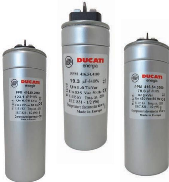
The capacitors making up the new **MONO Long Life Plus 4In** series are made using elements wound with the PPMh film and housed in metal cases with metal lids. The parts are assembled by crimping to ensure perfect airtightness of the system and efficient operation of the overpressure safety device.
