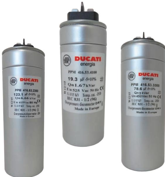
The capacitors making up the series **MONO Long Life 4In** are manufactured using elements wound with the PPMh film and housed in metal cases with metal lids. The parts are assembled by crimping to ensure perfect airtightness of the system and efficient operation of the overpressure safety device.
